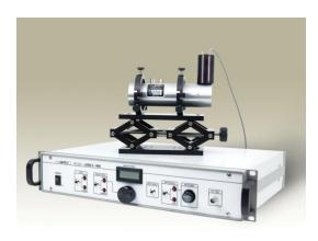
The LASS-II (Laser Amplitude Stabilization System) is an electro-optic feedback loop designed to reduce amplitude variations commonly associated with most gas lasers. This system is capable of significantly enhancing the signal/noise ratio of the laser over a much broader bandwidth than typical optically coupled current modulation of the plasma tube. Both an internal and external reference input is provided, allowing analog programming of the laser throughput. This is particularly convenient for
