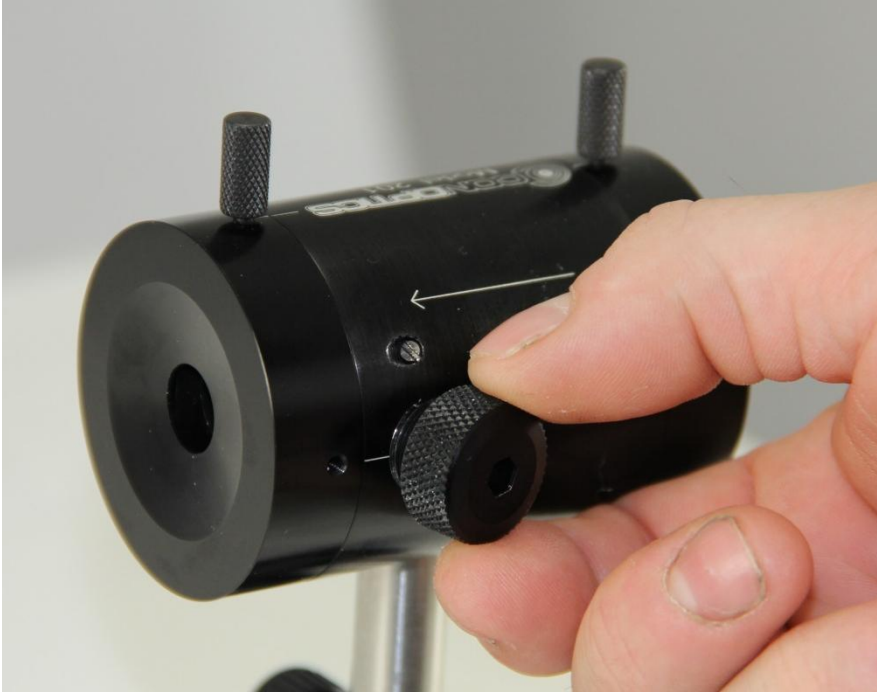
Beam Stop installed on Left side
